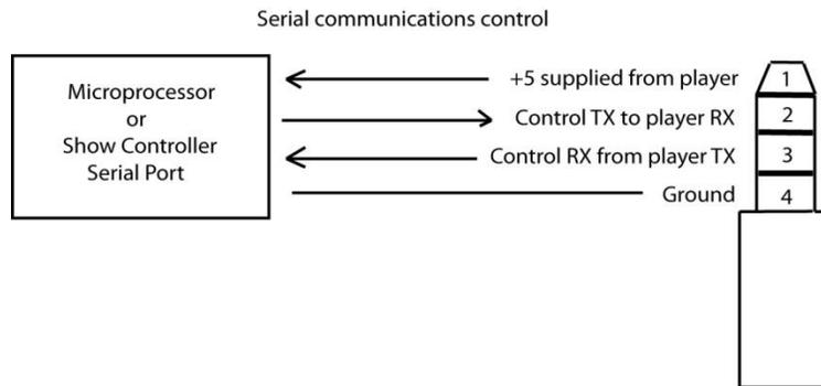
You can also use the included A/V cable in the I/O port. Use the Red RCA to send commands to the Sprite®, the yellow RCA for the Sprite® to report back to your control, and the white RCA for 5V power from the Sprite®. We suggest you cover the unused RCA plugs with electrical tape to avoid shorting the power supply and burning the internal fuse.
