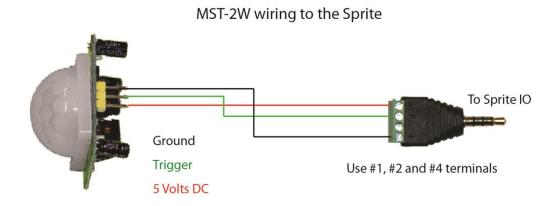
You can attach the 3 wires to the MST-2W in a few different ways.
