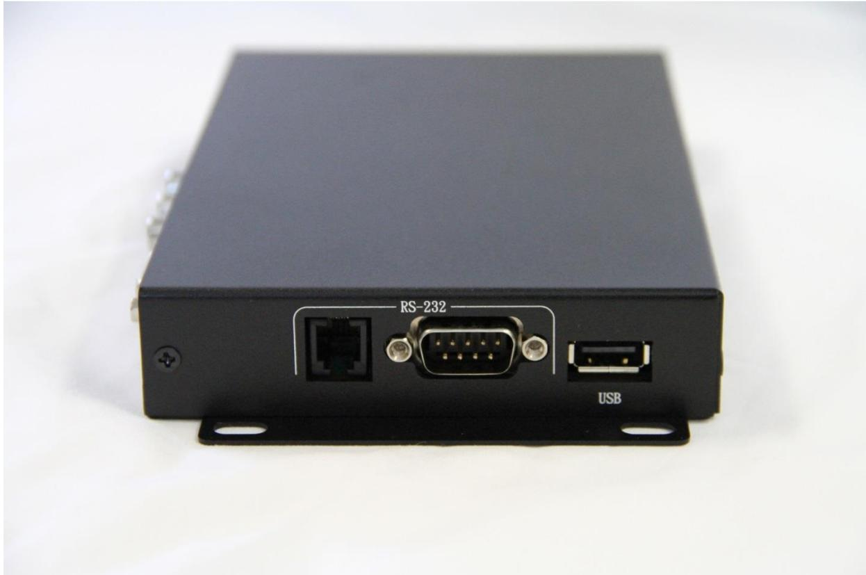
We use the RJ 9 port to connect the DV-68K, TK-69K or other control device.
