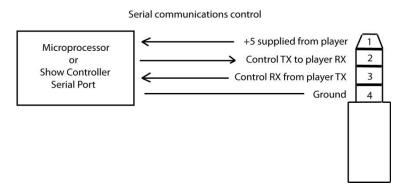
You can also use the included A/V cable in the I/O port. Use the Red RCA to send commands to the Sprite<sup>®</sup>, the yellow RCA for the Sprite<sup>®</sup> to report back to your control, and the white RCA for 5V power from the Sprite<sup>®</sup>. We suggest you cover the unused RCA plugs with electrical tape to avoid shorting the power supply and burning the internal fuse.
