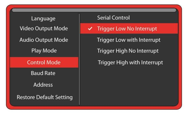
Select **Serial Control** to use an 8X78 input expander or external show control device or micro controller like a PIC, Atmel, Arduino, Raspberry Pi, or etc. using serial communications.
